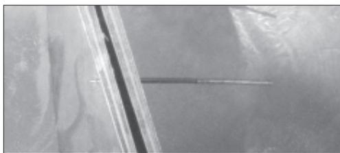
Fig. 28–14. Lancejet perforation of 0.75-inch plywood. MBA photo.
