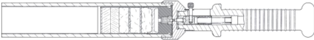
Fig. 28–97. 40mm threaded launcher loaded with triplex Stun-Bag cartridge. MBA drawings.
