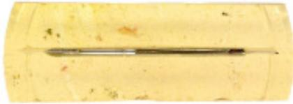
Fig. 28–21. Encapsulated 1.5mm Lancejet, sectioned. Actual size.
