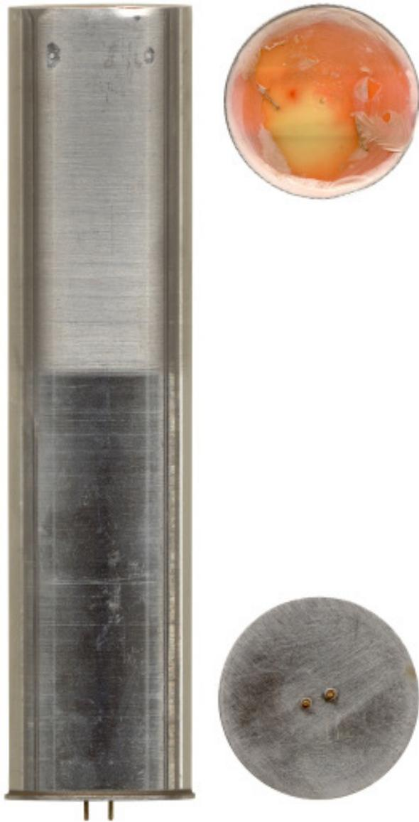
Fig. 28-103. MBA unknown electric initiated round with RR-129 dimensions. Actual size.
