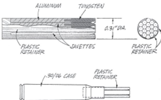
Fig. 28–25. Experimental .30-06 Javette-launching cartridge.
