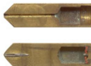
Fig. 28–42. M1 electric Javette cartridge sections. Actual size.
