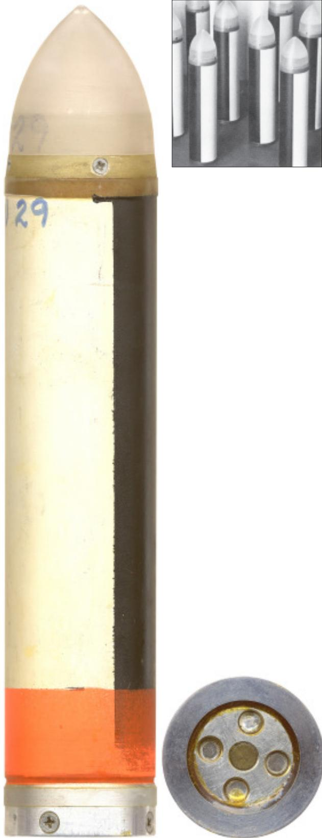
Fig. 28-95. 40mm Type I cloud seeding rocket and MBA photo.
