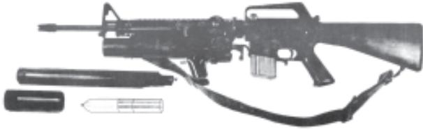
Fig. 28-92. MBA 30mm rocket adapter for M16 rifle and XM148 grenade launcher. MBA photo.
