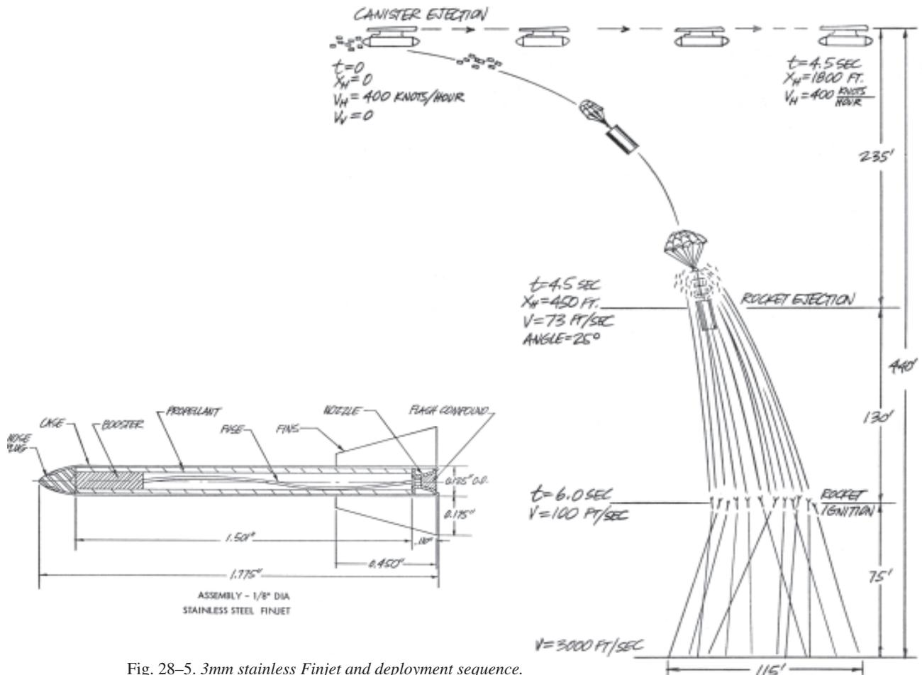
Fig. 28-5. 3mm stainless Finjet and deployment sequence.
