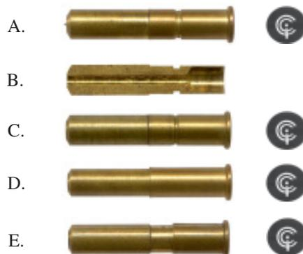
Fig. 28–49. Extended-Adapter .22 Javette rounds. (A) Snapped primer, Javette point at muzzle. Possible dummy for demonstration. (B) Factory section of adapter with no internal stainless hypodermic tube barrel. (C) Snapped primer, hypodermic tube. (D) Unsnapped primer, no cannellure, hypodermic tube. (E) Solid adapter (no bore) dummy in .22 Short case.
