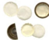
Fig. 28–46. Olin BWP electric primer with flash paper propellant. Actual size.
