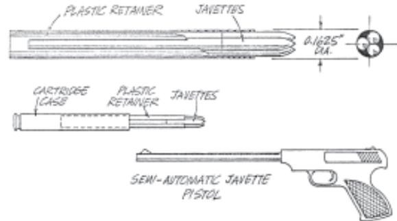
Fig. 28–26. Experimental .25-caliber Javette-launching cartridge.
