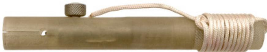
Fig. 28–73. Experimental MBA 13mm flare launcher. Actual size.
